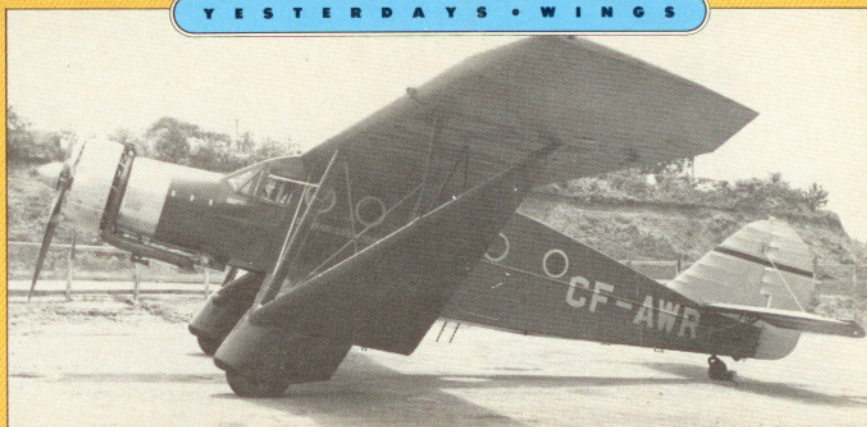
The Aircruiser was the last of the line that started with the Roma. The landing-gear fairings and the tail shape were the obvious changes; the significant ones were wing flaps and a controllable-pitch propeller.
